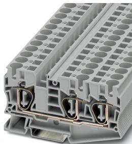
Feed-through terminal block, nom. voltage: 1000 V, nominal current: 57 A, connection method: Spring-cage connection, number of connections: 3, cross section: 0.2 mm<sup>2</sup> - 16 mm<sup>2</sup>, AWG: 24 - 6, width: 10.2 mm, color: gray, mounting type: NS 35/7,5, NS 35/15
