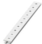
Marker for terminal blocks, Strip, white, labeled, can be labeled with: CMS-P1-PLOTTER, horizontal: U, V, W, N, GND, U, V, W, N, GND, mounting type: snap into tall marker groove, for terminal block width: 10.2 mm, lettering field size: 10.15 x 10.5 mm, Number of individual labels: 10
